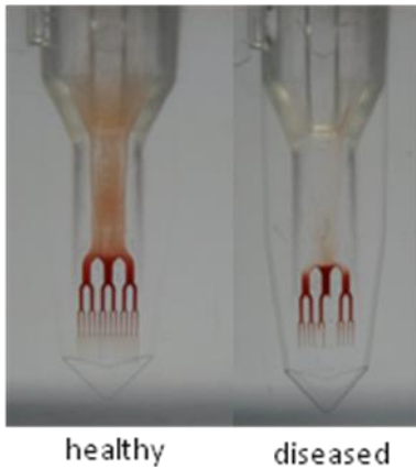
Figure 4. ESR measurement in cartridge. Left side healthy (negative sample), right side diseased (positive sample). The sedimentation rate of the diseased sample is increased.
