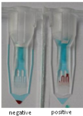
Figure 3. Agglutination assay for bloodgroup determination. Left side no agglutination (negative sample), right side agglutination (positive sample).
